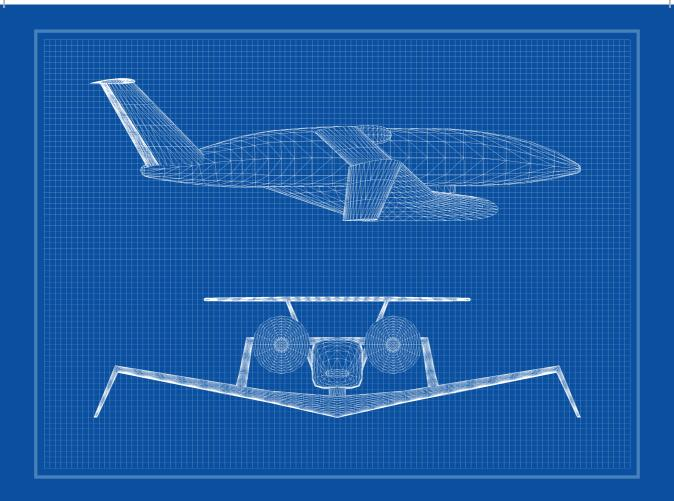
AIRSHIP envisions an innovative use of a known transportation mean: flying ships. Such vehicles (also known as ekranoplans or wing-in-ground -WIG- vehicles) are designed and built to take advantage of the ground effect, allowing these crafts to fly with enhanced lift and reduced drag, which translates into better energy efficiency and lower environmental impact, without sacrificing any of the advantages of conventional airborne transportation.
